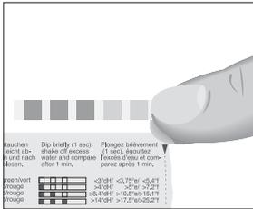
You can find out what the water hardness is by using the Aquadur® test strip supplied as standard.
